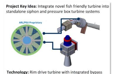
and additively manufactured honeycomb guide vanes
